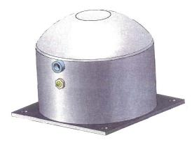
The MP-11 is used to provide gauge pressure sensors with an ambient reference that has no moisture/humidity that can cause errors and/or sensor failure. Once connected to the reference tube of a pressure sensor the MP-11 allows for a change in barometric pressure with very little error. The advantage of the MP-11 is zero maintenance. There are no filters or desiccant to check or change.
